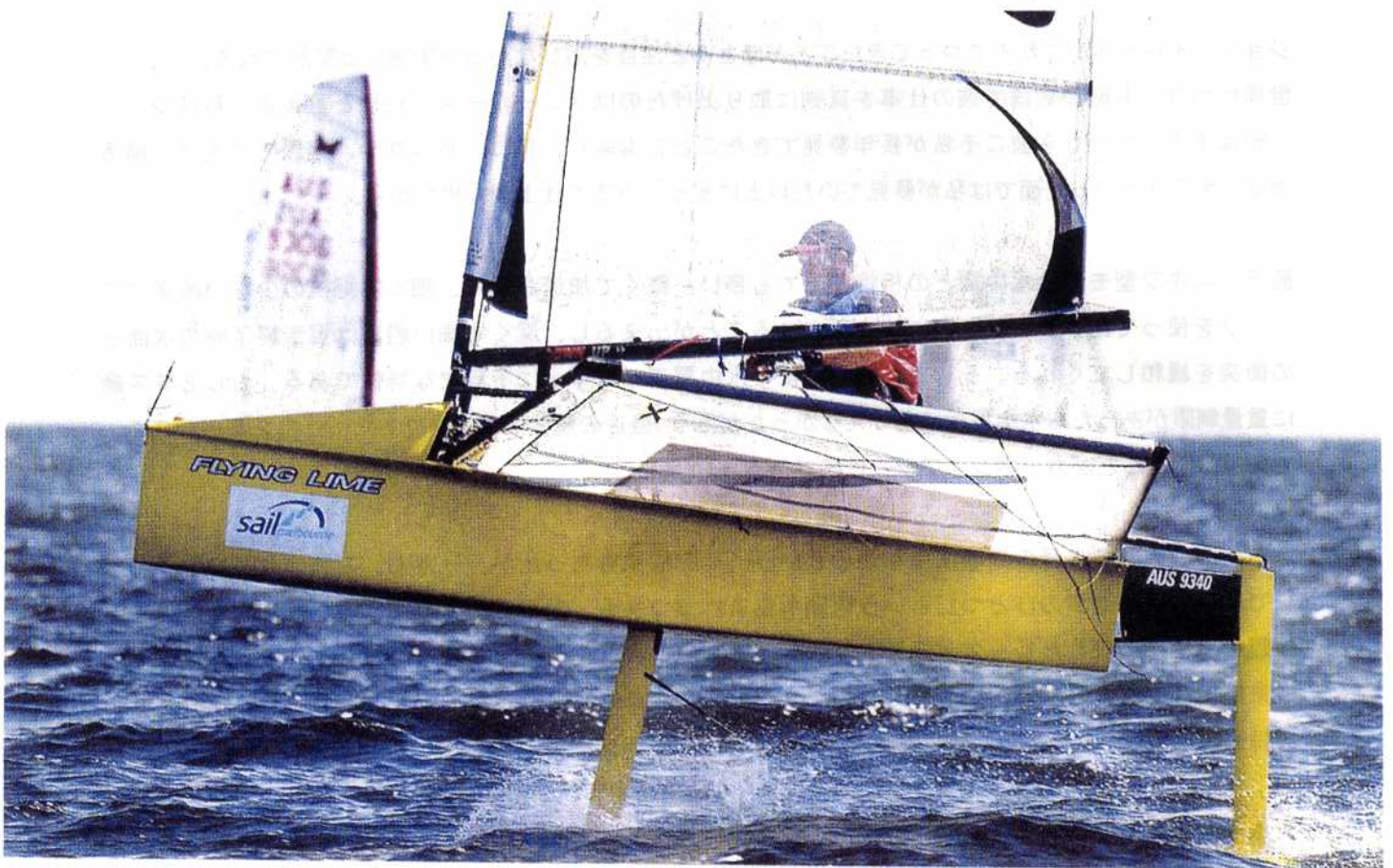
Above: bi-foiler pioneer John Ilett from Perth finished 13th at this year's championship but took plenty of satisfaction from seeing Veal ( left ) dominate the event using his latest production hull and foils. Note Ilett's latest fin – rather than bow – mounted height sensor
