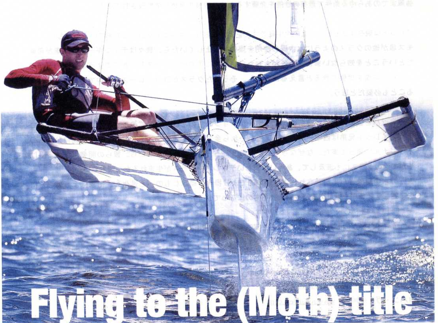
Above: bi-foiler pioneer John Ilett from Perth finished 13th at this year's championship but took plenty of satisfaction from seeing Veal ( left ) dominate the event using his latest production hull and foils. Note Ilett's latest fin – rather than bow – mounted height sensor
